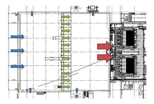
• When the doors to the tipping hall are opened to allow lorry movements, air is drawn in via the open doors supplemented, where required, by smaller quantities of air drawn through the louvres at the back of the tipping hall.
